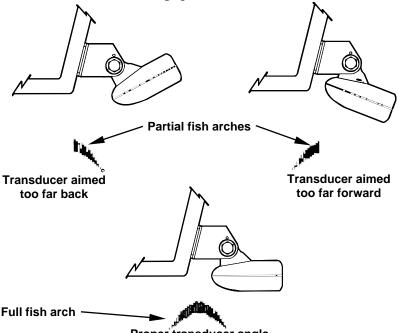
Proper transducer angle
